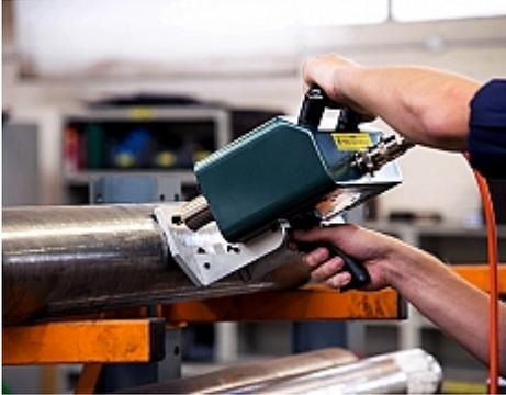
The Pryor PortaDot Range provides a fast and portable method of dot-peen marking, otherwise known as dot marking. It is ideal for marking permanent alphanumeric, logo or 2D barcode information onto immobile, large or heavy components and is often used in rail, oil and gas, foundry and construction applications.
